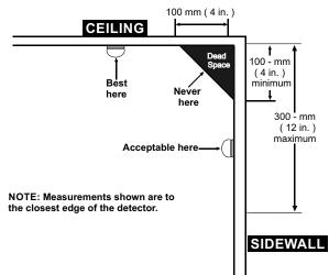
KEEP SMOKE DETECTORS OUT OF DEAD SPACES WHERE WALLS MEET THE CEILING
